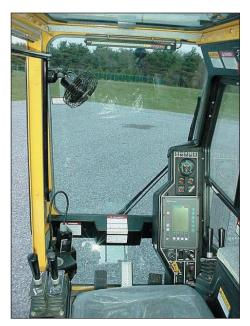
All steel fabricated superstructure cab has padded acoustical lining for sound suppression, safety glass and excellent visibility under close working conditions.
