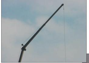
26 ft. - 45 ft. telescoping swingaway extension with offset up to 30° maximizes up and over capacity.
